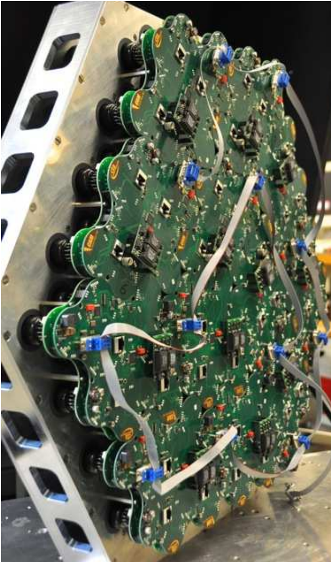
FIG. 7.2 – Rear view of the 144-pixel prototype showing the control boards.
