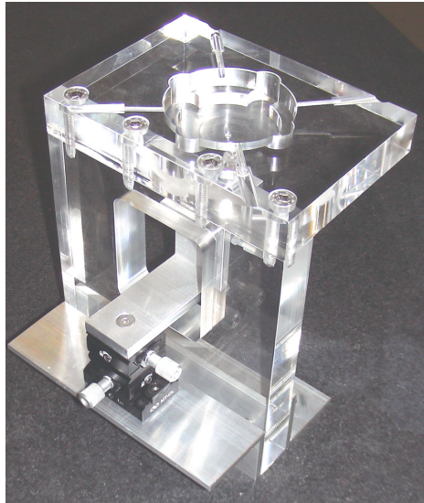
Figure 14.8: Custom built sample holder for the Institute of Physiology.
