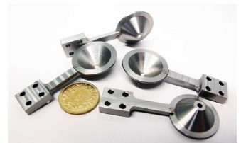
Dedicated sample holders for the low energy electron point source (LEEPS)
