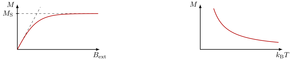
(a) Plot of M vs. B_{\text{ext}} . Curie's law holds for low B_{\text{ext}} .
