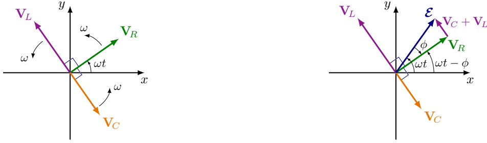
(a) Each reactance adds a rotating phasors. (b) The vectorial sum of the reactances is the EMF \mathcal{E} .
