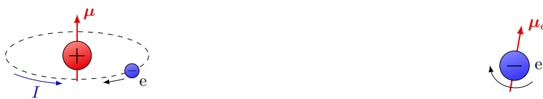
(a) Electrons orbiting around the atom form a current, giving the atom a magnetic moment \mu .
