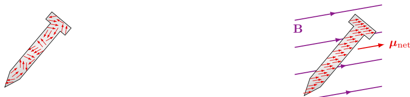
(a) No field: The nail has microscopic domains (not to scale in figure) with magnetic moments pointing in random directions.
