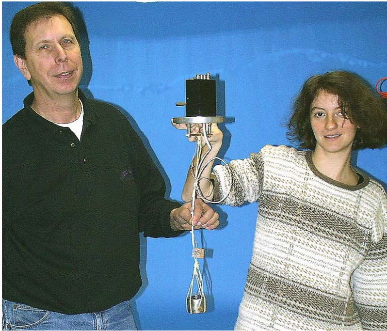
A first "bare" HPGe detector
