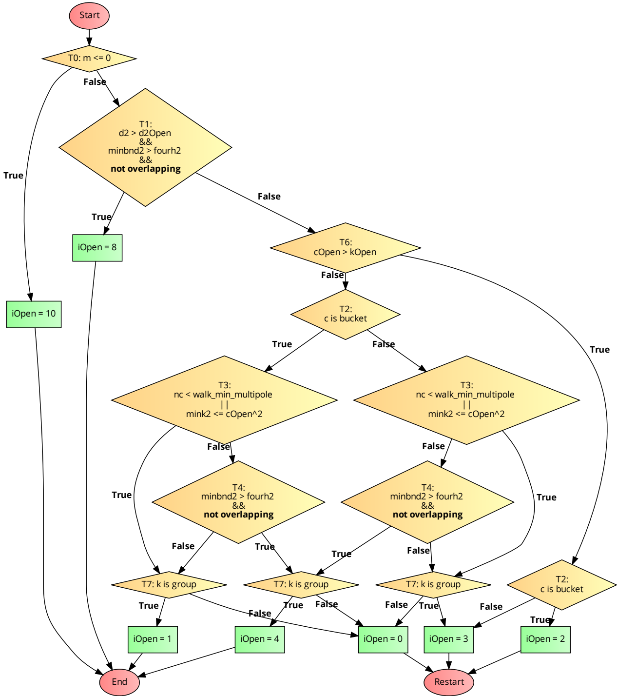
Figure 2: Decision tree of the opening criterion. The sink cell for which the force is to be calculated is called k, while the source cell is called c. The new SPH overlap tests are highlighted in bold.
