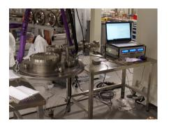
Test setup for the evaporation of the wavelength shifting reflectors for the LEG-END experiment (group Baudis).
