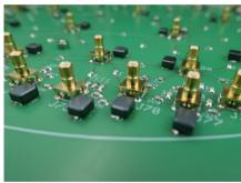
Detail of a circuit that simulates the dynamics of wave propagation in a hyperbolic space (group Neupert).
