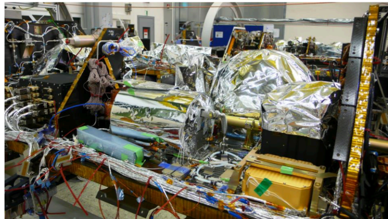
LRI fully mounted on FM1 During functional testing
