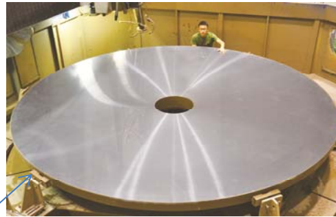
SiC mirror of 4 m aperture
