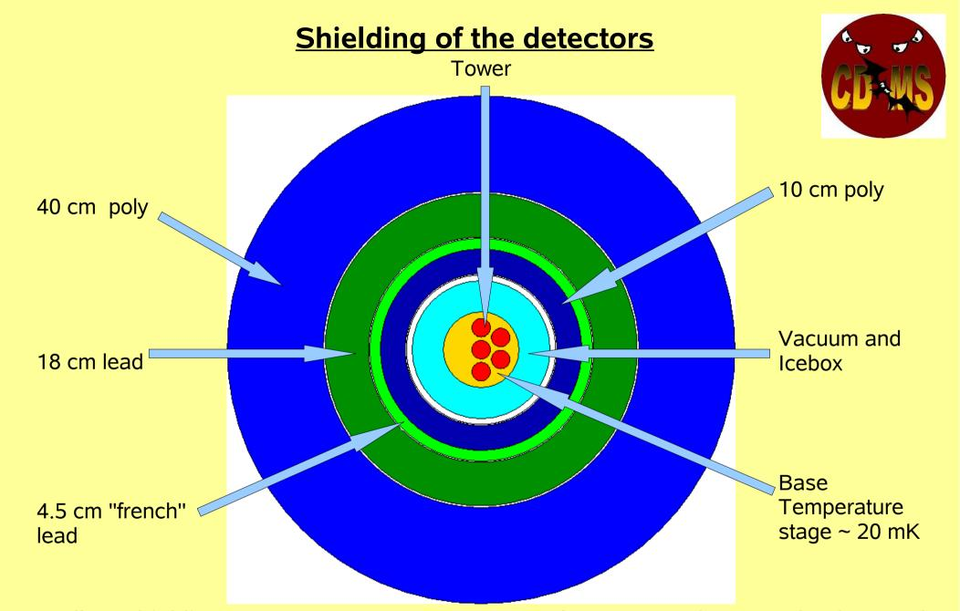
Excellent shielding necessary to suppress external neutron and gamma background. But contaminations of our internal materials are a source of gamma backgrounds.
