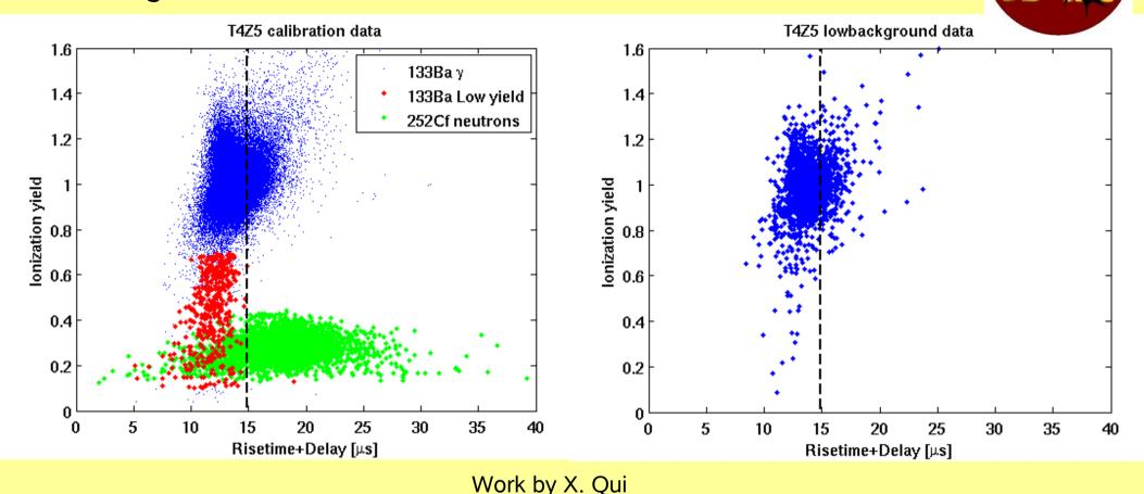
Timing cut **chosen** at a level to contribute ~0.5 events total leakage to WIMP candidates.
