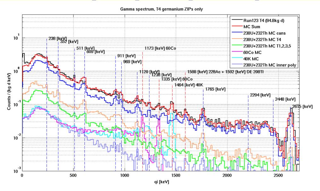
MC simulations of known background sources match the observed spectra very well. There are **no** hints for additional contaminations from unexplained spectral lines.
