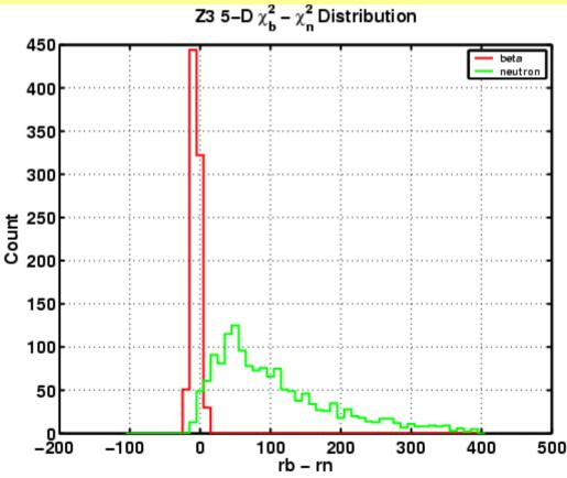
Cut can be set to exlude all betas while maximizing the neutron acceptance.
