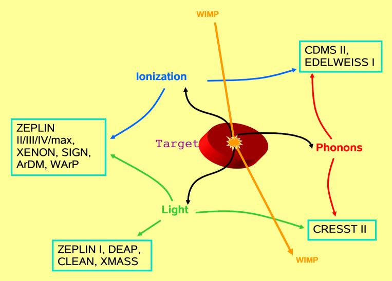
Several channels can be used to disriminate background from signal for low energetic recoils ( $\sim$  < 100 keV).
