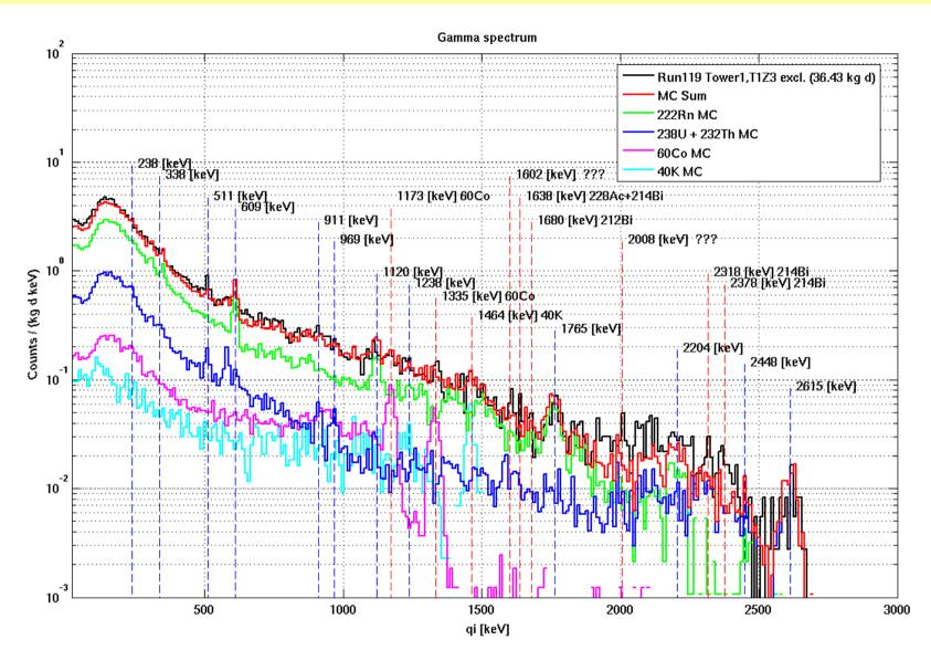
Natural radioactivity of our materials is causing our gamma background. MC simulations of known background sources matches the observed spectra very well.
