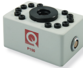
Figure 17: Test box to put the sample holder used for the determination of the sheet resistance at room temperature [28]
