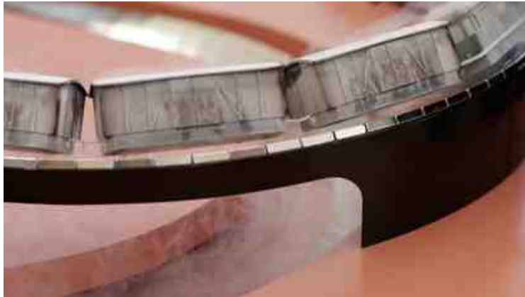
Figure 1: Train levitated by superconductors on a magnetic trail
