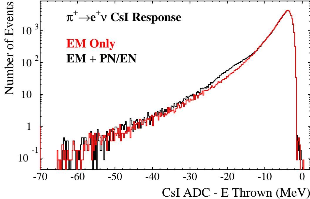
GEANT4 Calculations including photonuclear and electronuclear interactions, compared with electromagnetic-only showers, with source  $\pi \rightarrow e\nu$  and  $\mu \rightarrow e\nu\bar{\nu}$  positrons.
