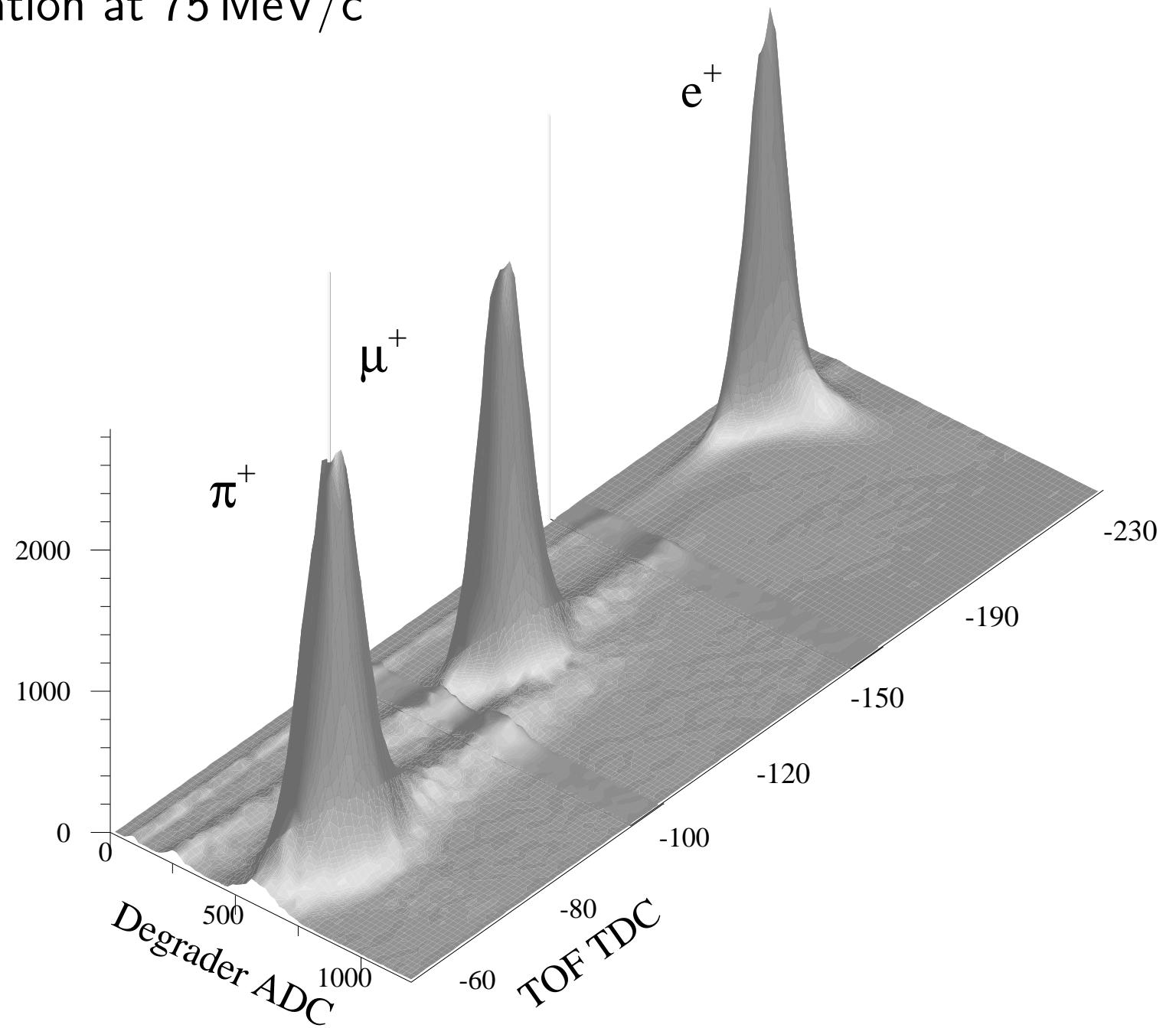
Separation between  $\pi$ -stop and  $\pi \rightarrow \mu$  events in the Target
