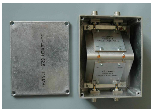
Figure 2.3: Duplexer built for the SCOPES NMR-spectrometers.
