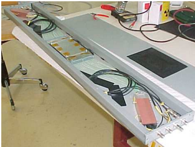
Figure 2: Picture of the test detector with the active area in the center of the open box and the wls fibres which are connected to the photomultipliers.
