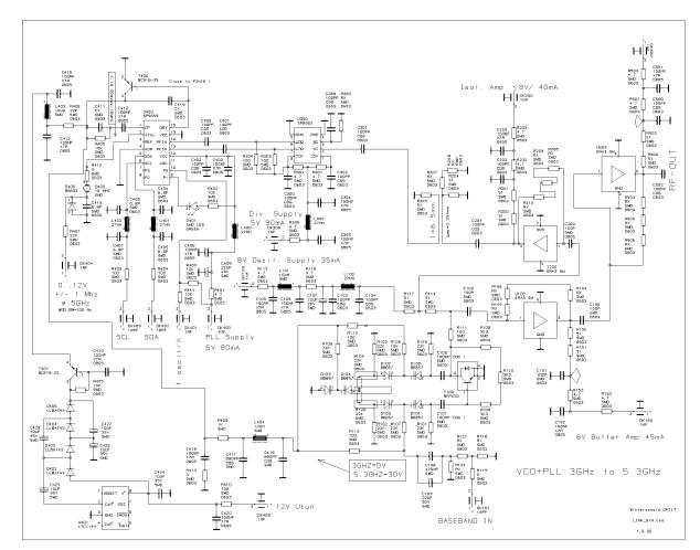
In short, from DC to 7GHz there is nothing but 5GHz for 80dB down. Phase noise is about -90dBc @ 100kHz, Sidebands caused by 16MHz XTAL are also 80dB down. (see spectrum plot below). Nice for a Spectrum Analyzer swept LO, but too complicated, too many parts for LINK application.
