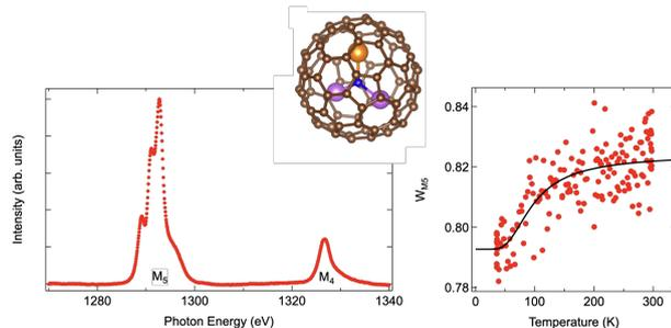
Resonant x-ray absorption spectrum at the Dy  $M_{4,5}$  edge of  $\text{DySc}_2\text{N@C}_{80}$  on a Pt(111) surface (left). The spectral weight of the  $M_5$  edge  $W_{M_5}$  depends on the temperature and indicates the onset of endohedral rotation at about 90 K. The solid line is a thermodynamic model that describes the endohedral motion (right panel). The inset depicts one endohedral fullerene molecule with a diameter of 1.1 nm. Dysprosium yellow, nitrogen blue. Data R. Sageshashi *et al.*
